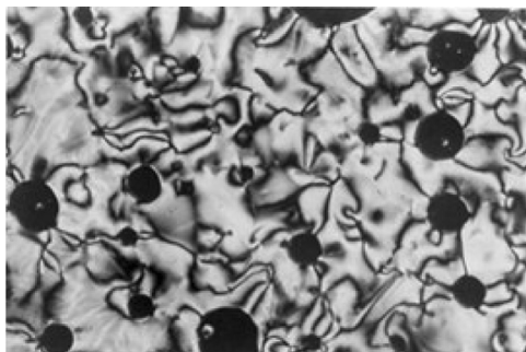
FIGURE 7 Smectic C schlieren texture of 6-12 at 236°C.
